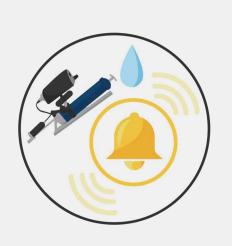
Use ultrasound equipment to apply lubricant once the lack of lubrication alarm has been reached. Apply lubricant until dB falls to the baseline level.
