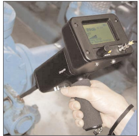
Figure 3. Some ultrasonic translators can log test results such as decibel and frequency readings. The heterodyned signal can be used to record sound samples or to connect directly to vibration analyzers for detailed spectral or time series analysis.
